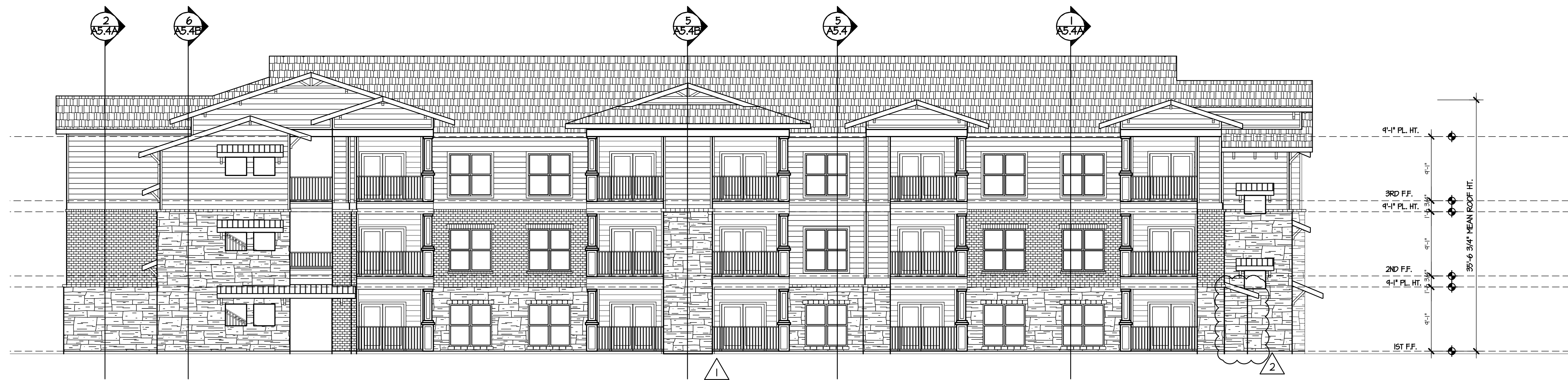
1 BLDG TYPE III - FRONT ELEVATION 1/8"
