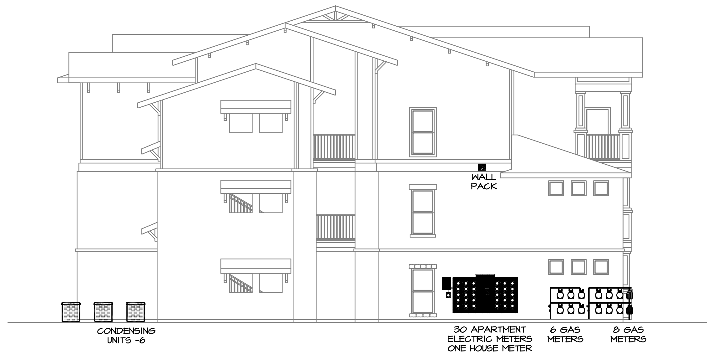
BUILDING TYPE III RIGHT ELEVATION - MEP
