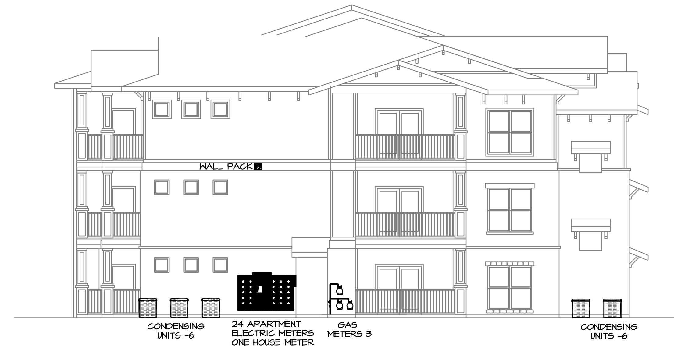
BUILDING TYPE II LEFT ELEVATION - MEP 1/8" = 1'-0"
