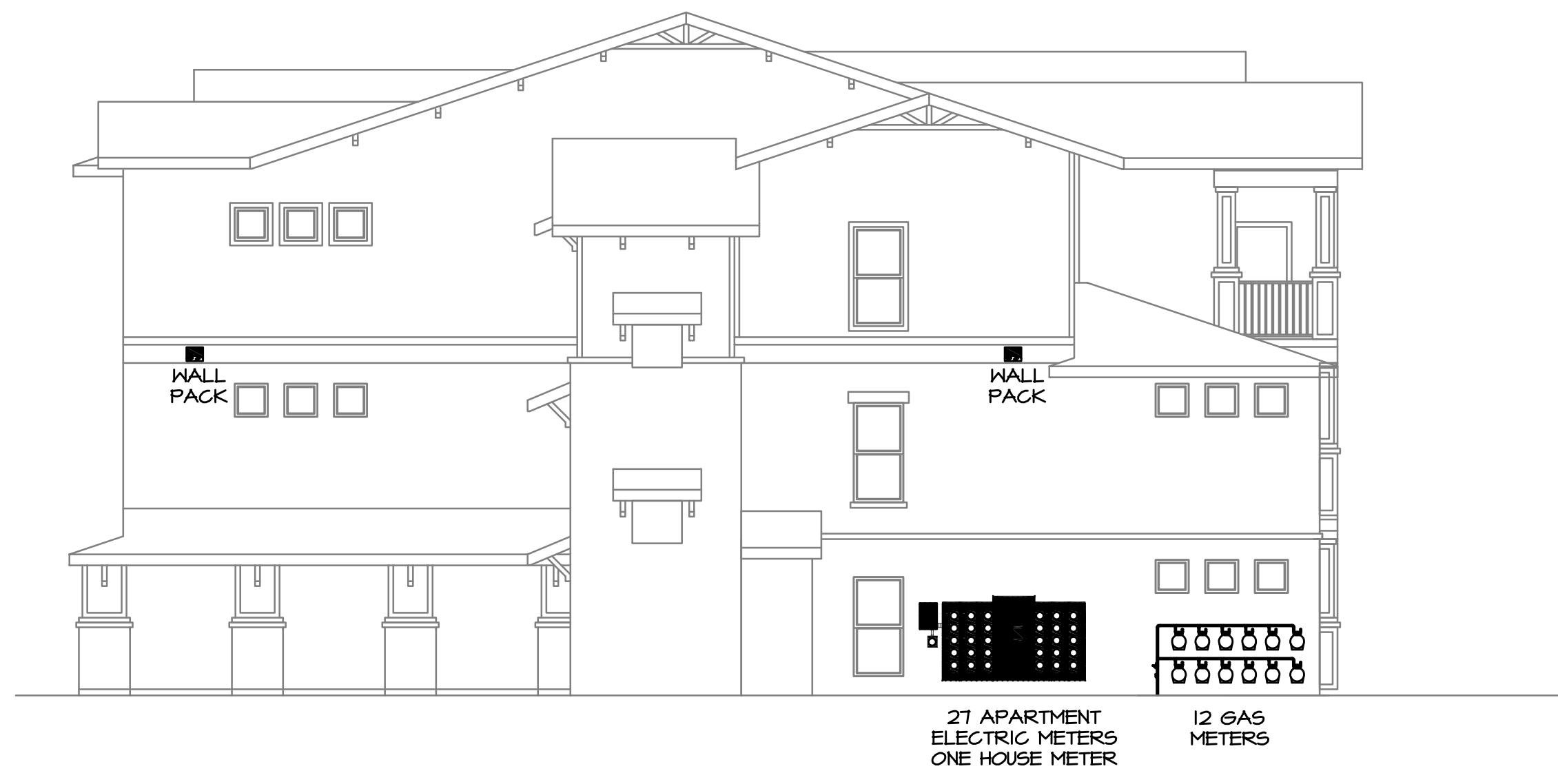
BUILDING TYPE IV RIGHT ELEVATION - MEP
