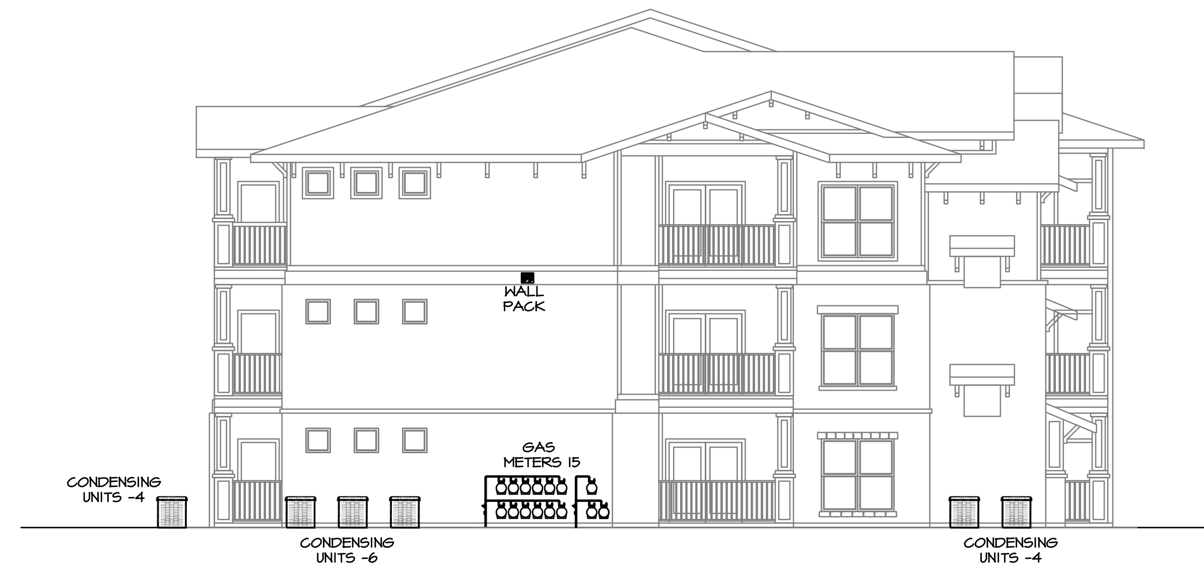
BUILDING TYPE I LEFT ELEVATION - MEP
