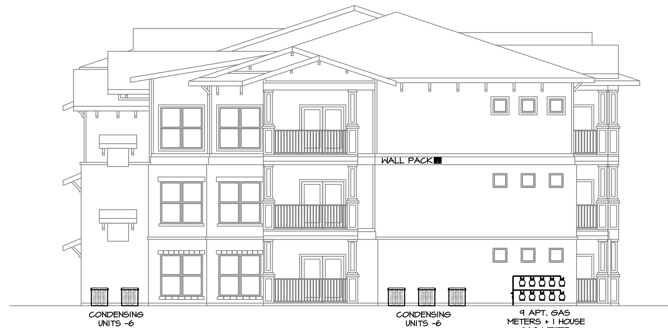
BUILDING TYPE II RIGHT ELEVATION - MEP 1/8" = 1'-0"
