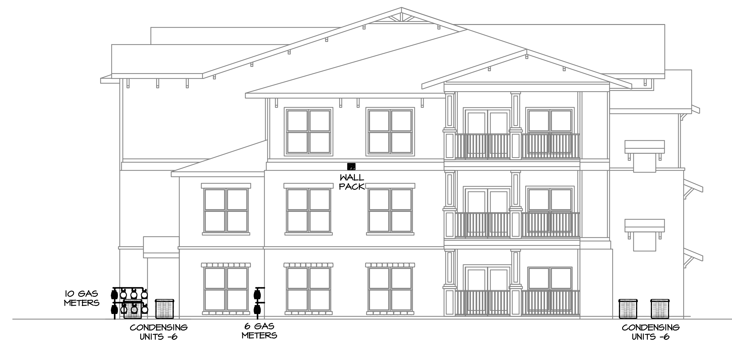
BUILDING TYPE III LEFT ELEVATION - MEP
